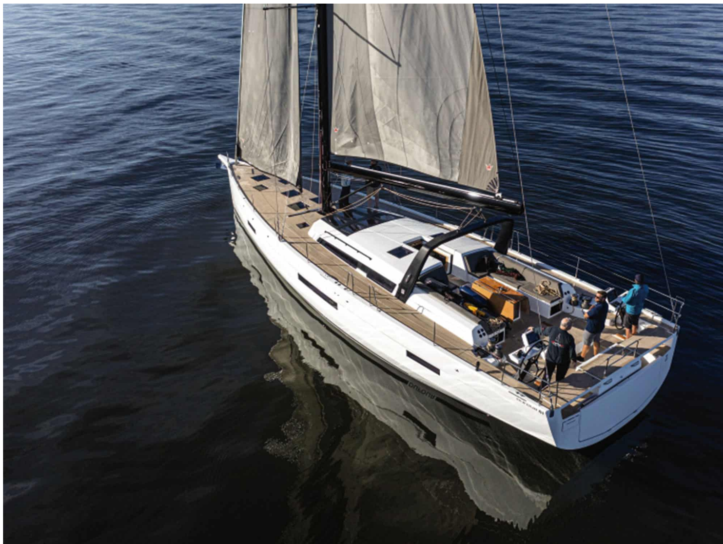
The Dufour 61's mainsheet is anchored on a cockpit arch. Jon Whittle
